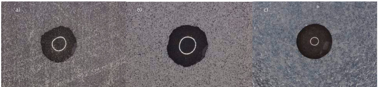
Figure 4: EOS PA 2200 parts with a water drop of 20 \mu L volume on differently treated surfaces. a) Water drop on colored EOS PA 2200 ( r=4,5\text{mm} ), b) on PSS treated and colored EOS PA 2200 ( r=3,8\text{mm} ), c) on VFS treated and colored EOS PA 2200 ( r=2,7\text{mm} ).
